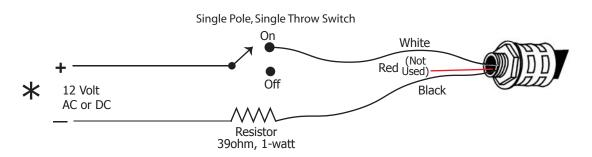
\* The LAD pigtail 2.1mm coaxial adapter can be used to connect to a GXF-10 Littlite power supply.
